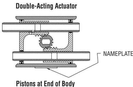
**IMPORTANT:** Note the relative location of the shaft teeth and the piston assembly’s rack teeth. The above figure is viewed when looking at the top of the actuator.
