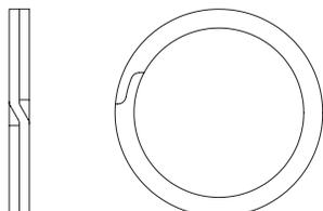
To remove this clip, engage the lower end of the ring with a flat blade screwdriver. Using another flat blade screwdriver push the top end of the clip in the opposite direction. As the clip I.D. expands, lift the clip from the shaft. The installation of a new clip would be the above steps in reverse and ensuring that the edges of the clip are properly seated in the shaft groove.
